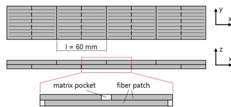
Figure 2: Structural FPP lamina with representative unit cell.
