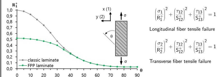
Figure 5: Tensile strength of unidirectional CFRP laminae as a function of the fiber orientation / off-axis angle  $\theta$ .
