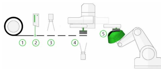
Figure 1: Schematic illustration of the FPP process: (1) feeding of fiber tape, (2) (laser-)cutting of tape in patches, (3) inspection of patches, (4) picking up and position check of patches, (5) placing the patches onto the forming tool. [1]
